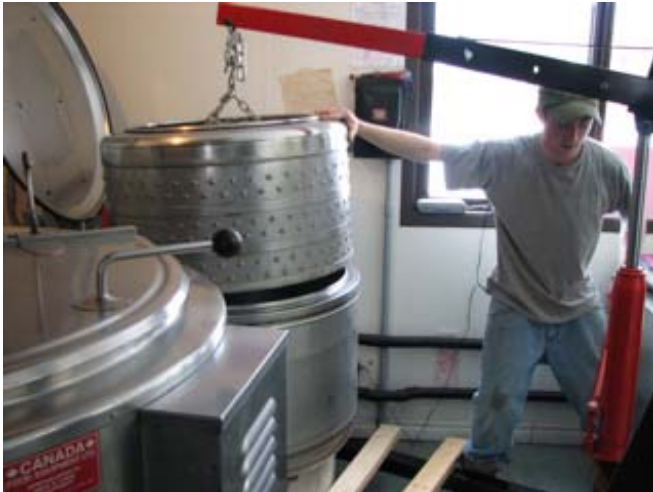
2006 spring–Jake Dixon cranking cooked soybeans out of the kettle with a cool custom colander (under sheet of stainless steel that is used as a ramp between kettle and centrifuge).
