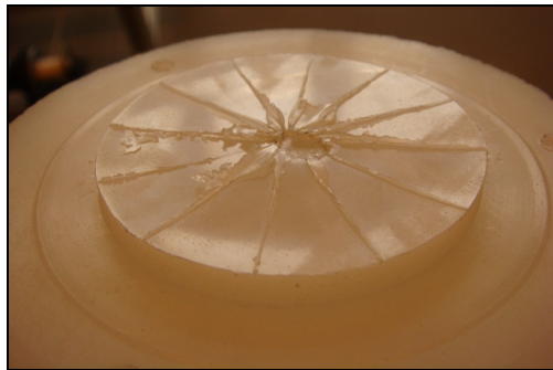
Figure 5.2: Typical "Pizza Valve" Puncture Test Result
