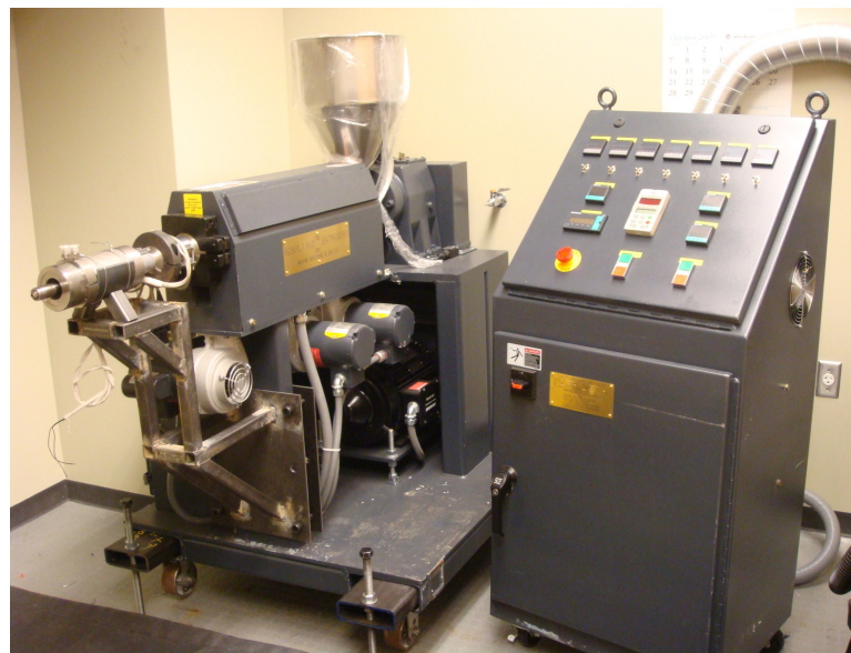
Figure 3.16: Extruder and Accompanying Melt Injection Equipment of the EARFM Experimental Setup
