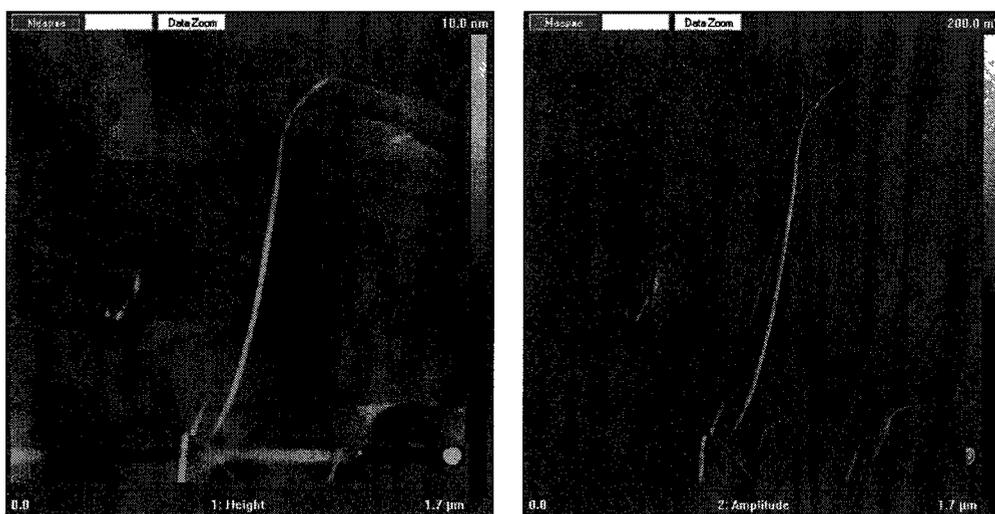
Figure 4.18: AFM images of compound **4.16** aged for 4 days in methanol and diluted to 0.2 mg/mL. Sample was cast on a mica substrate.
