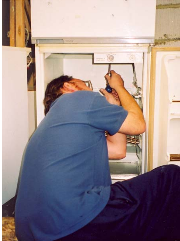
Figure 6.6 Doug replacing a thermostat
