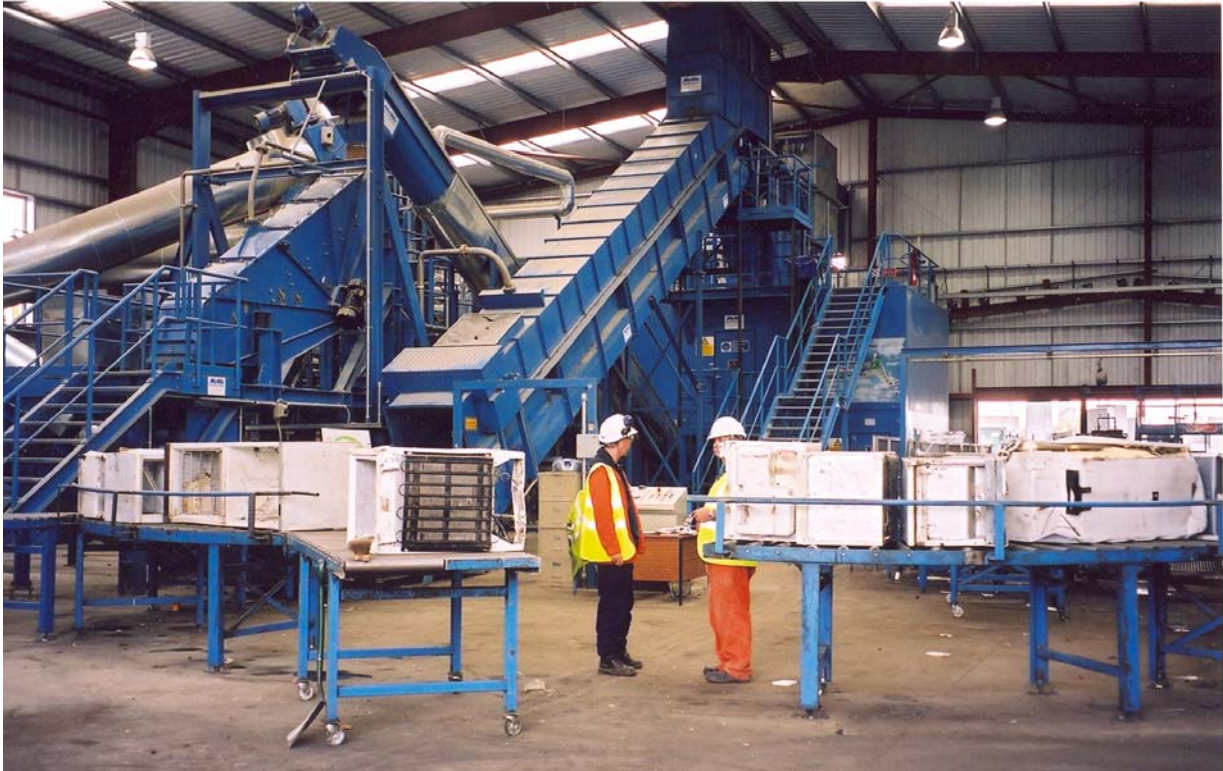
Figure 6.12 On route to the sealed ‘cyclone chamber’ to be broken down
