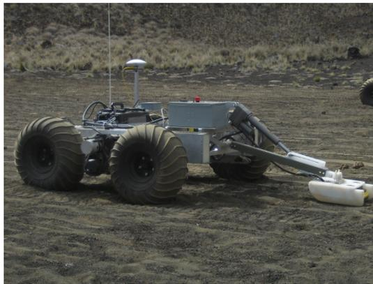
**Figure 2.3:** Location of the rover motors between fore and aft wheels. Photo courtesy of Terence Fu.
