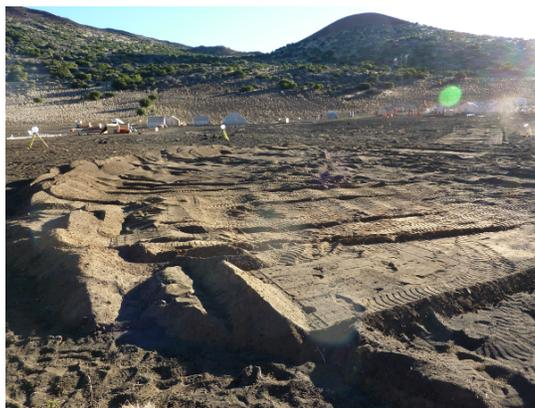
**Figure 3.5:** Example of an excavation pass with unacceptable oscillations. A flat excavation pass (foreground) is contrasted by an oscillating excavation pass (midground) during the Mauna Kea deployment. Photograph courtesy of Kenneth Law.
