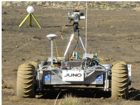
**Figure 2.2:** Rear view of a rover showing the battery compartments partially-obstructed by the walking arm suspension. Battery compartment covers can be identified by their CSA stickers. Photograph courtesy of Paul Grouchy.
