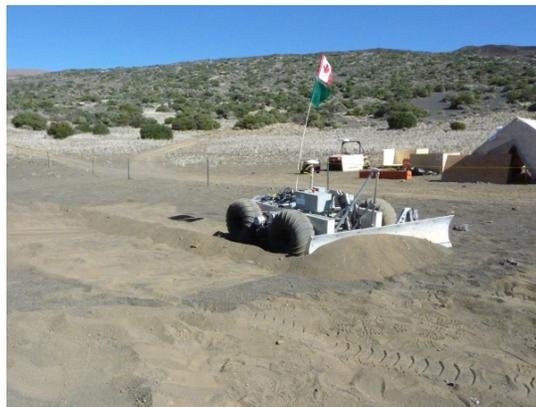
**Figure 6.1:** *Athos* testing the digging controller during the Mauna Kea deployment. Photograph courtesy of Kenneth Law.
