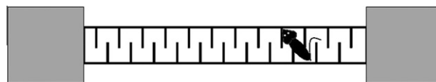
Fig. 2. FlexMaze apparatus. The FlexMaze consists of a long (8 × 80 cm) transparent corridor with regularly spaced staggered doors that force lateral flexion with exploration. Each end of the maze is attached to a neutral, beige compartment (15 × 15 cm) by a 6 × 6 cm opening. The 4-cm-wide doors are staggered on alternating sides and are placed every 4 cm.
