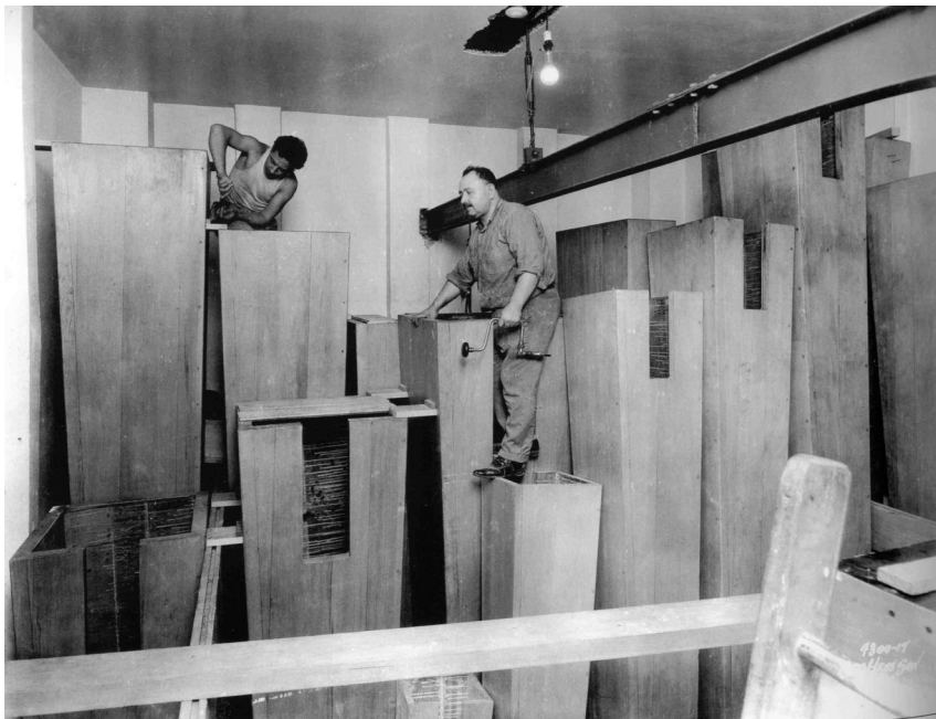
Figure 14. Building the 32-foot Diaphone, Atlantic City
