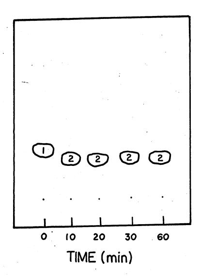
mixture. Its R<sub>f</sub> value and color reaction are shown in Table II. The rate of chemical reduction of phloroglucinol was also followed spectrophotometrically. A shift in the absorption peak from 268 mµ to 278 mµ was found after ten minutes incubation and this new peak at 278 mµ did not disappear when the reaction mixture was incubated for 1 hour.
