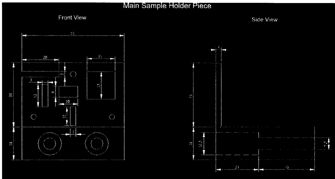
Figure 3.2: Design details of the main sample holder which contains various holes through which the laser beam enters. Three threaded holes are used for screwing in the back pressure plate. All measurements are in mm.
