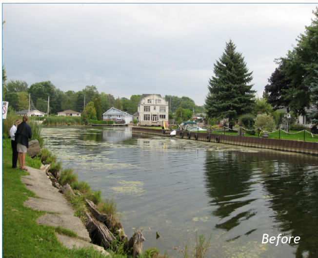
Walter Drive Erosion Control Project Before and After - approximately 630 m of shoreline was rehabilitated through bioengineering techniques including placement of river stone, fascines and live stakes, and the planting of 250 native trees and shrubs.
