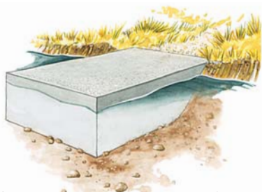
Concrete piers are expensive and environmentally destructive.
