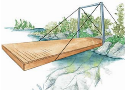
A tower and thick cables keep a suspension dock up in the air.
