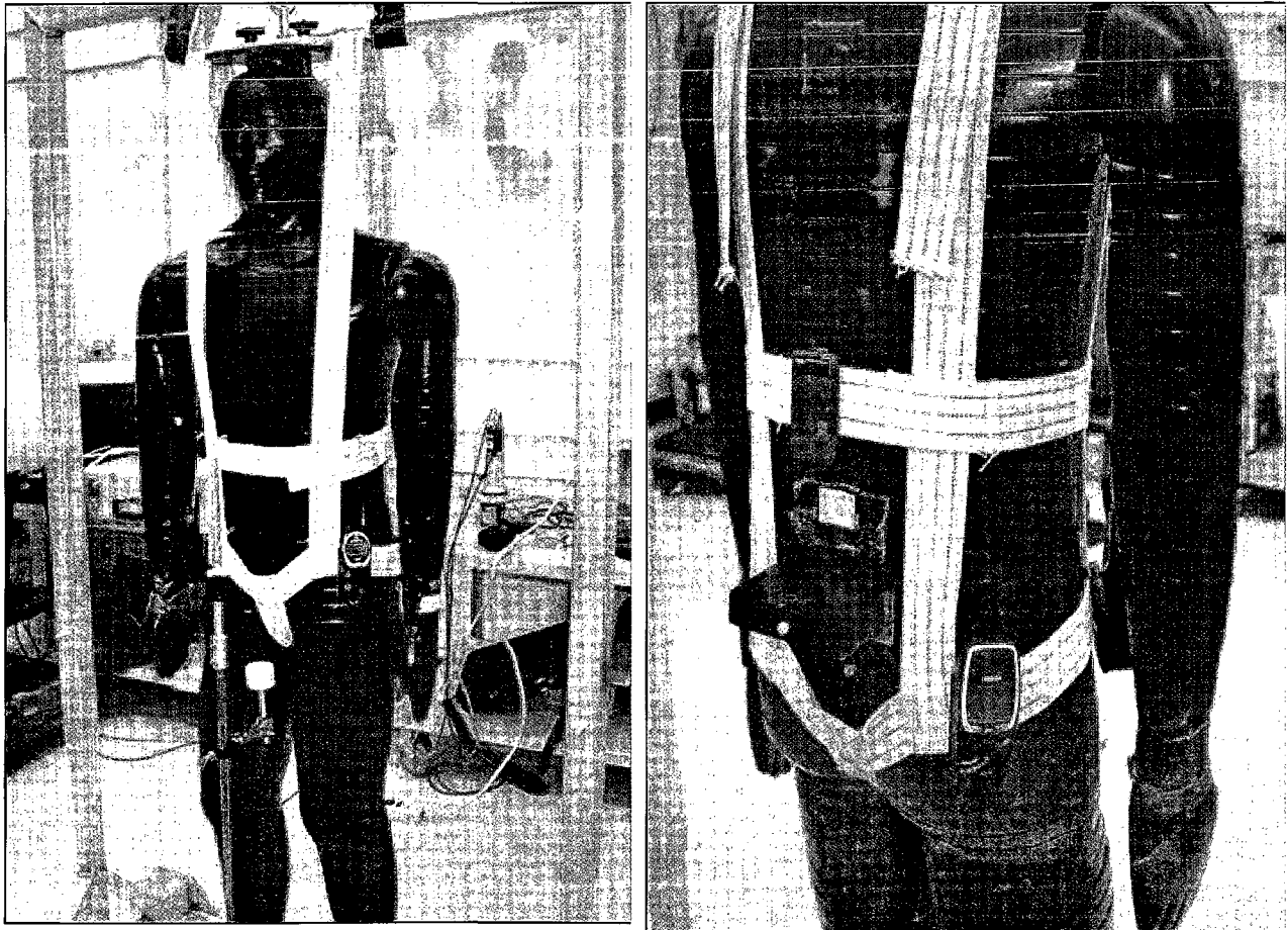
Figure 20. Cellular phones and electronic dosimeters affixed to DRDC Ottawa's anthropomorphic phantom for RED simulation trials.
