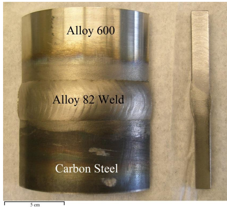
Figure 19 – an Alloy 82 dissimilar metal weld joint between parent materials of Alloy 600 and carbon steel (shown on the left). The weld was cut axially to reveal the cross-section of the weld (shown on the right).
